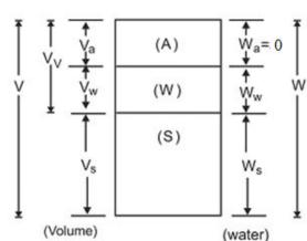
Three Phase diagram (Partially saturated)
